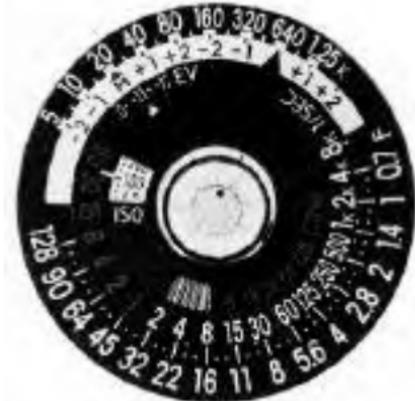
This 20 indicates the exact center point of the luminance range. In the same condition, install Lumigrad and when standard reflectivity of 18% is measured, this means that the dial scale will indicate 20. When determining exposure by using the Lumisphere or Lumidisc,
