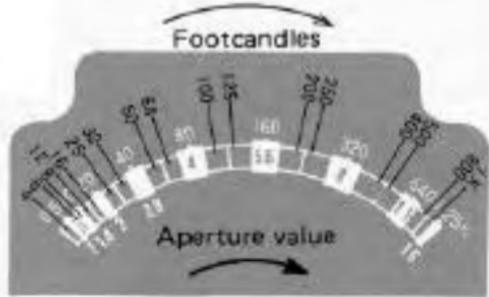
intermediate values for shutter speed and aperture scale
